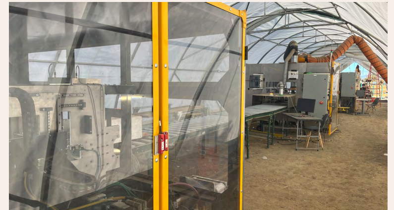
Urban Machine's processing line is almost 120 feet long and 30 feet wide. Four different robot arms move around each other in order to pick the lumber free of metal nails and other fasteners.
